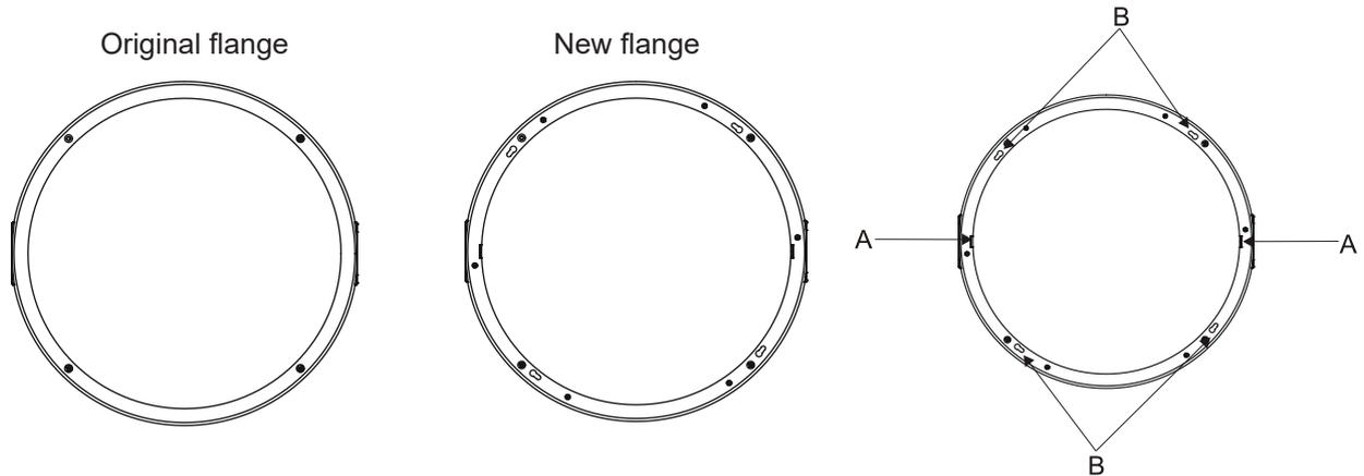
3. Place the top hat (1) on the head (5), press locks (2) and turn the top hat counter-clockwise until it snap into slots (B) in the flange.
