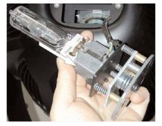
5. Replace the lampholder assembly in its original position and refasten the two screws "A" which were previously removed.
