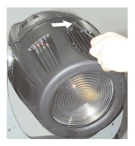
2. Lift the housing to gain access to the internals of the fixture.
