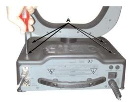
1. Loosen the screws on the cover of the base of the unit, as shown in the diagram below, using an appropriate screwdriver, thereby removing the cover completely and allowing access to the internal components of the base of the **iWash Halo**.
