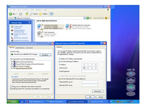
After network configuration, type the IP address of the DigitalSpot 7000 DT in address line in your Windows explorer window. Use this format **ftp:**// **2.X.X.X** / (e.g. ftp://2.236.2.88/- see picture below).
