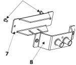
6. Snap the two insulating washers with outer diameter of 10mm (10) into SDI/ASI connectors holder (8) and fasten this holder on the rear panel (3) with two screws M3x10 (9). The SDI/ASI cables (11) have to aim at the bottom of the fixture base.
