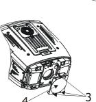
**4.** Place the long (short) throw optic module (5) instead of the module of the glass cover (4) and secure it by the 3 quarter-turn fasteners (6).
