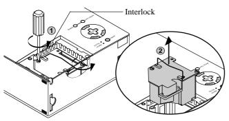
3. Insert a new lamp housing until the lamp housing is plugged into the socket.
