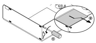
2. Loosen the two screws securing the lamp housing until the screwdriver goes into a freewheeling condition. The two screws are not removable.
