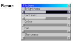
Provides access to controls for your image. Use the "Select" button on the projector cabinet or the remote control to highlight the menu for the item you want to adjust.
