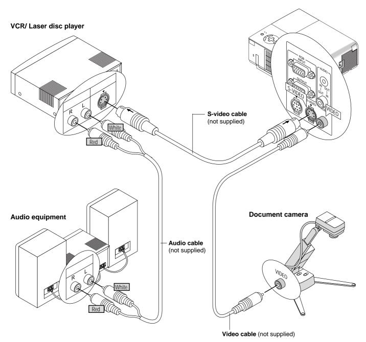
Use common RCA cables (not provided) to connect your VCR, laser disc player or document camera to your projector. To make these connections, simply:
