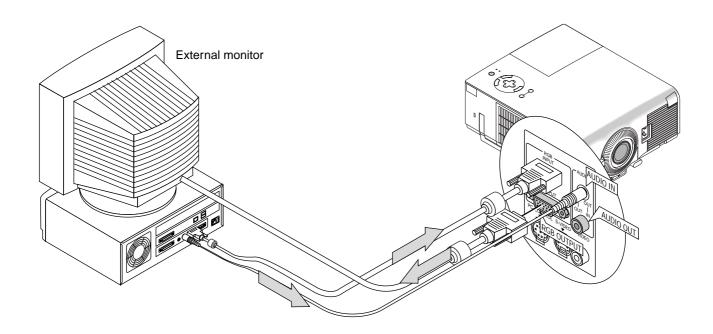
You can connect a separate, external monitor to your VT440/VT540 to simultaneously view on a monitor the image you're projecting. To do so: 1. Turn off the power to your projector, monitor and computer.
