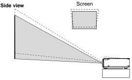
(There is approximately 10 degrees of up and down adjustment for the front of the projector.)
