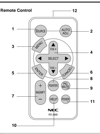
**NOTE:** Remove the transparent insulation tape before use. See page E-34 for battery installation.
