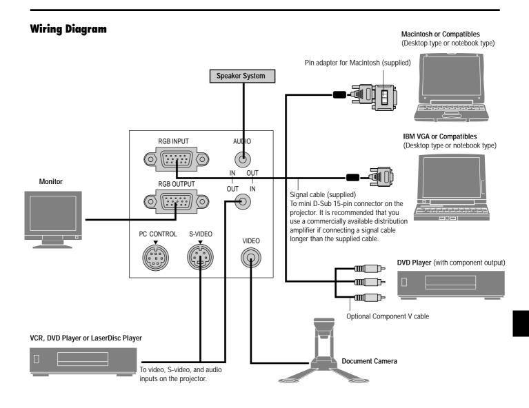
**NOTE:** When using with a notebook PC, be sure to connect between the projector and the notebook PC before turning on the power to the notebook PC. In most cases signal cannot be output from RGB output unless the notebook PC is turned on after connecting with the projector.
