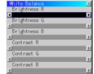
This allows you to adjust the white balance. Brightness for each color (RGB) is used to adjust the black level of the screen;
