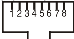
RJ-45 socket (front view):
