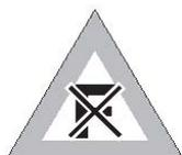
**This symbol indicates that the unit must not be laid on an inflammable surface or in any case must be kept away from naked flames**
